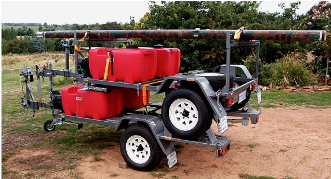
Fig 9: Mast-trailers with ballast tanks, masts on top rack. Pic by Chris Tidemann.
